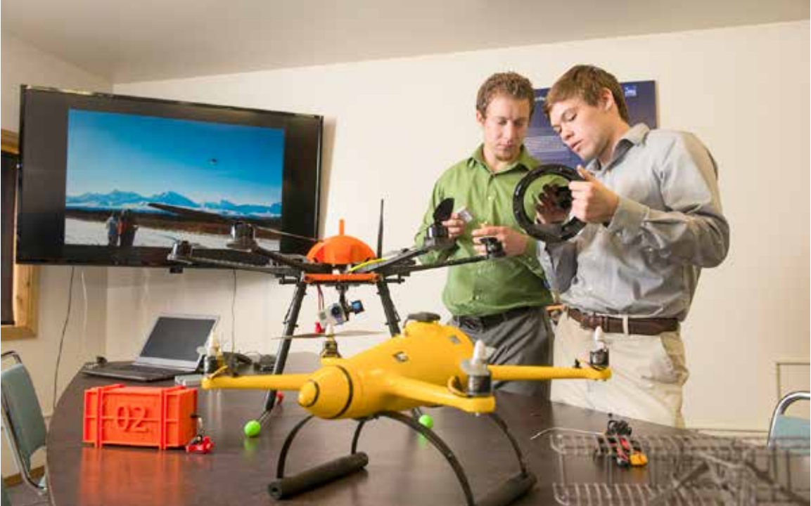
Sam Vanderwaal, left, and Corey Upton determine how to install a camera and a video transmitter in a drone payload extension module. The black drone with an orange top on the table is a Ptarmigan UAS designed by NES staff; the yellow drone is an H20Copter.
